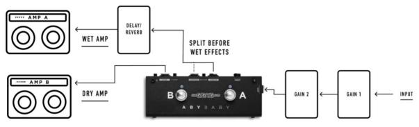
There are loads of different ways you can set this up, and the fact that you can reverse the relative phase, lift the earth, and easily select which output you want means that it will work as a signal splitter in any situation.
