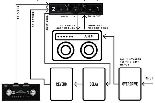
In this example the overdrive pedal is plugged directly into the front of the amp. The overdrive could be a boost, or any other pedal that you prefer in the front of the pre-amp. The idea here is that we're are getting the gain/distortion we need from the amps' pre-amp or by boosting into the pre-amp. From there the UnderLiner is connected to the amps fx loop with delay and reverb in the loop of the UnderLiner.
