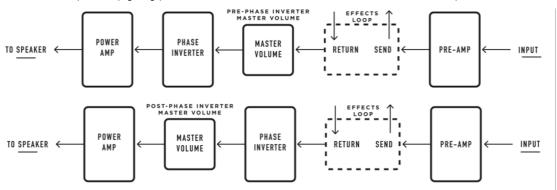
In some amps the overdrive is created by slamming the signal from the pre-amp into the phase inverter valve. In this scenario the UnderLiner will give you the option to reduce the signal driving the phase inverter giving you less distortion. The UnderLiner can give you 2 extra attenuated levels on top of the amps max gain level.
