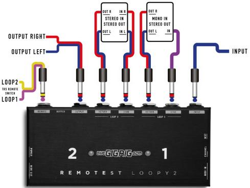
For a pedal that has a MONO input and a STEREO output, select M on the M/ST switch. In this setting the TIP is sent to both the TIP and RING on the loop sends.
