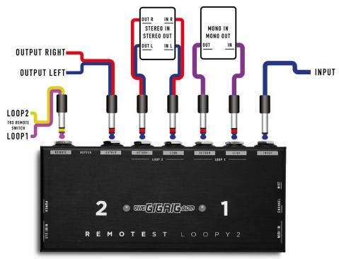
When mixing MONO and Stereo effects, you need to remember that as soon as you put a TRS in any of the send and returns, every send and return will need a TRS connection. Pay special attention to the cable on the LOOP RETURN. If you want to be able to switch between combinations of MONO and STEREO effects the output of the MONO effect needs to go both to the left and right return of the REMOTEST LOOPY2 Loops. The easiest way to achieve this is with a MONO to TRS/STEREO cable.
