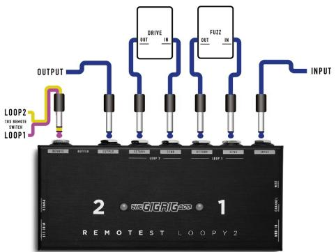
ST/M Switch setting for a standard MONO set-up is ST. The ST/M switch only applies when you are using a MONO input with TRS cables in the effect loops.
