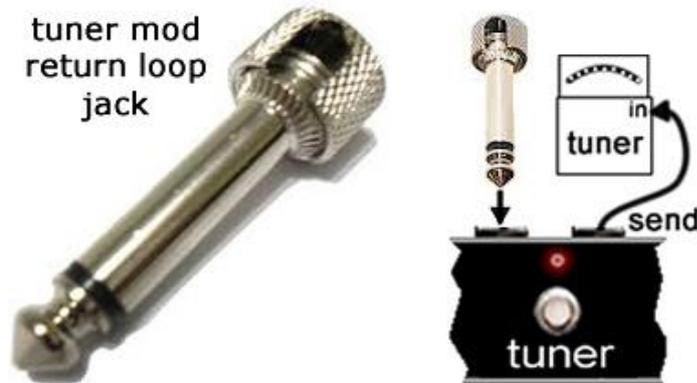
The jack included with your **QuarterMaster** is a short-circuited jack that you can use to turn a standard true bypass loop into a silent tuner send option.
