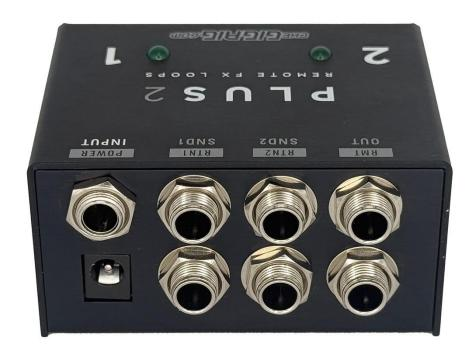
INPUT — Signal input. If you are placing PLUS2 at the start of your signal chain this would be your guitar input. You can place Plus2 anywhere in your signal path
